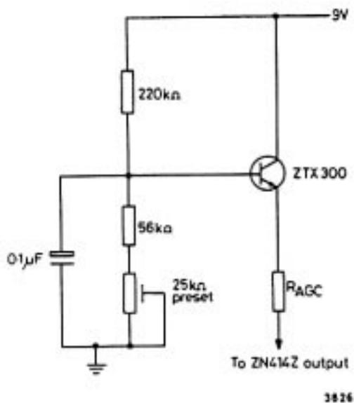
Current consumption is virtually that which is taken by the ZN414Z ( $0.3\text{mA}$ )
