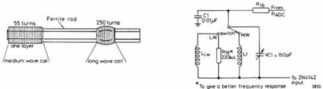
Coil winding details and waveband selection
